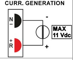
Measuring a 0..11 V voltage signal (internal impedance 100 kOhm)
