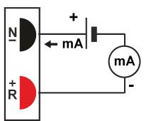
Current generator 0..21 mA Voltage generator 0..11 V with loop powered by an (minimum load impedance: 1 external power unit ( Vmax: 24 Vdc).
