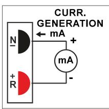
Current generation 0..21 mA with loop powered by Test-4 (Maximum Load Impendance 400 Ohm).
