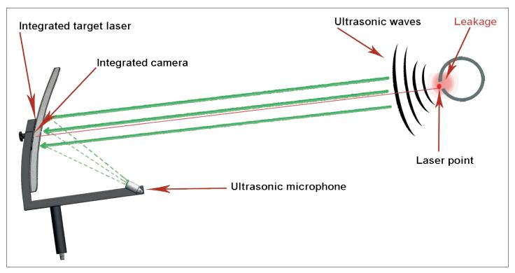
By bundling the ultrasonic waves in the parabolic mirror, even the smallest leaks of 0.8 I / min (ca.  $8 \in \text{p.a.}$ ) at a distance of up to  $10 \dots 15 \text{ m}$  can be localized with pinpoint accuracy ( $\pm 15 \text{ cm}$ ). The shape of the parabolic mirror ensures that only ultrasonic waves of the targeted leak are evaluated. Noise is reduced to a minimum.
