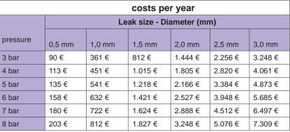
Table: Leakage costs within one year in case of operation 24 h/365 days, calculated with compressed air costs of 1.9 ct/Nm³.
