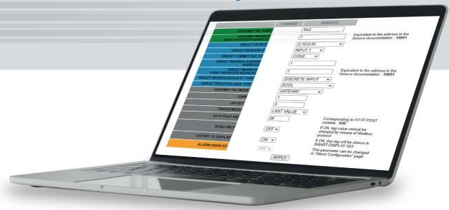
For more advanced configuration and operation requirements, particularly in terms of connectivity and control logics, SSD offers a Web Server through which remote configurability is assured and complete with the device from a specific IP address (e.g. http://192.168.90.101:8080)
