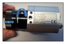
Figure 13: Inserting the lens
