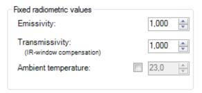
Figure 45: Adjustment of the emissivity in the software PIX Connect (menu Tools/ Configuration/ Device)
