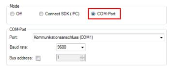
3. Select the baud rate that matches the baud rate of the other communication device. The other interface parameters are 8 data bits, no parity and one stop bit (8N1).
