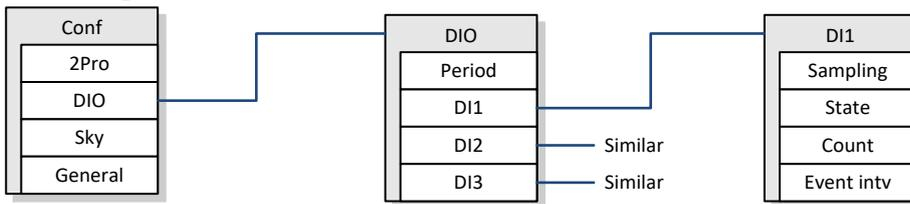
There is a common **Period** setting applying to all the digital inputs. With this period, the states and counts of the digital inputs are transmitted with the radio. In addition, there may be separate event transmissions as explained below. It is advisable that the analog period is a multiple of the digital period or vice versa, or they share the value, because then the transmissions stay in sync, allowing them to be combined in the same radio packet.
